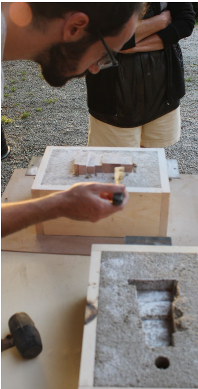
Fig. 2: Participants of the workshop preparing sand moulds for the aluminum casting exercise.
